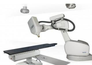
Several beam modifying accessories are available. Imaging systems are mounted on the Linac for better patient positioning. The system is fully computer controlled.
