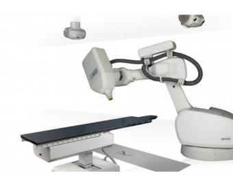
Several beam modifying accessories are available. Imaging systems are mounted on the Linac for better patient positioning. The system is fully computer controlled.
